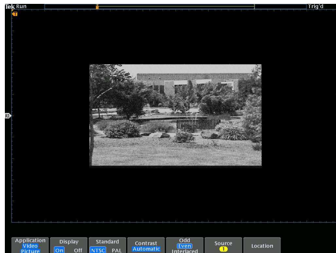
Viewing an NTSC video image. Video picture mode contains automatic contrast and brightness settings as well as manual controls.
